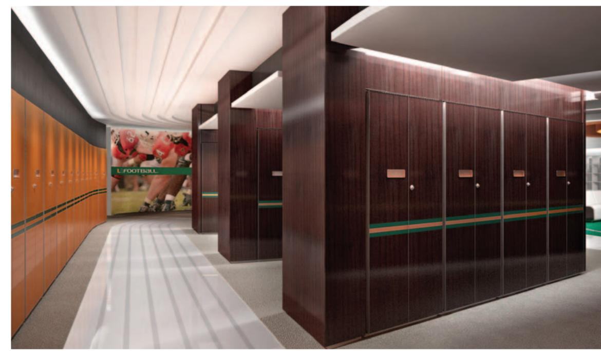
**The Lockers** We are proposing a re-thinking of the basic locker design based on both functional needs and our desire to create a more distinctive branded design. The first thing you will notice about the proposed locker design is that they have doors. This is designed to allow for dedicated ventilation to each individual locker. We have incorporated this method in other lockers and the result is a
